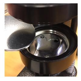
4. Place metal backing piece in tray, pin side down
